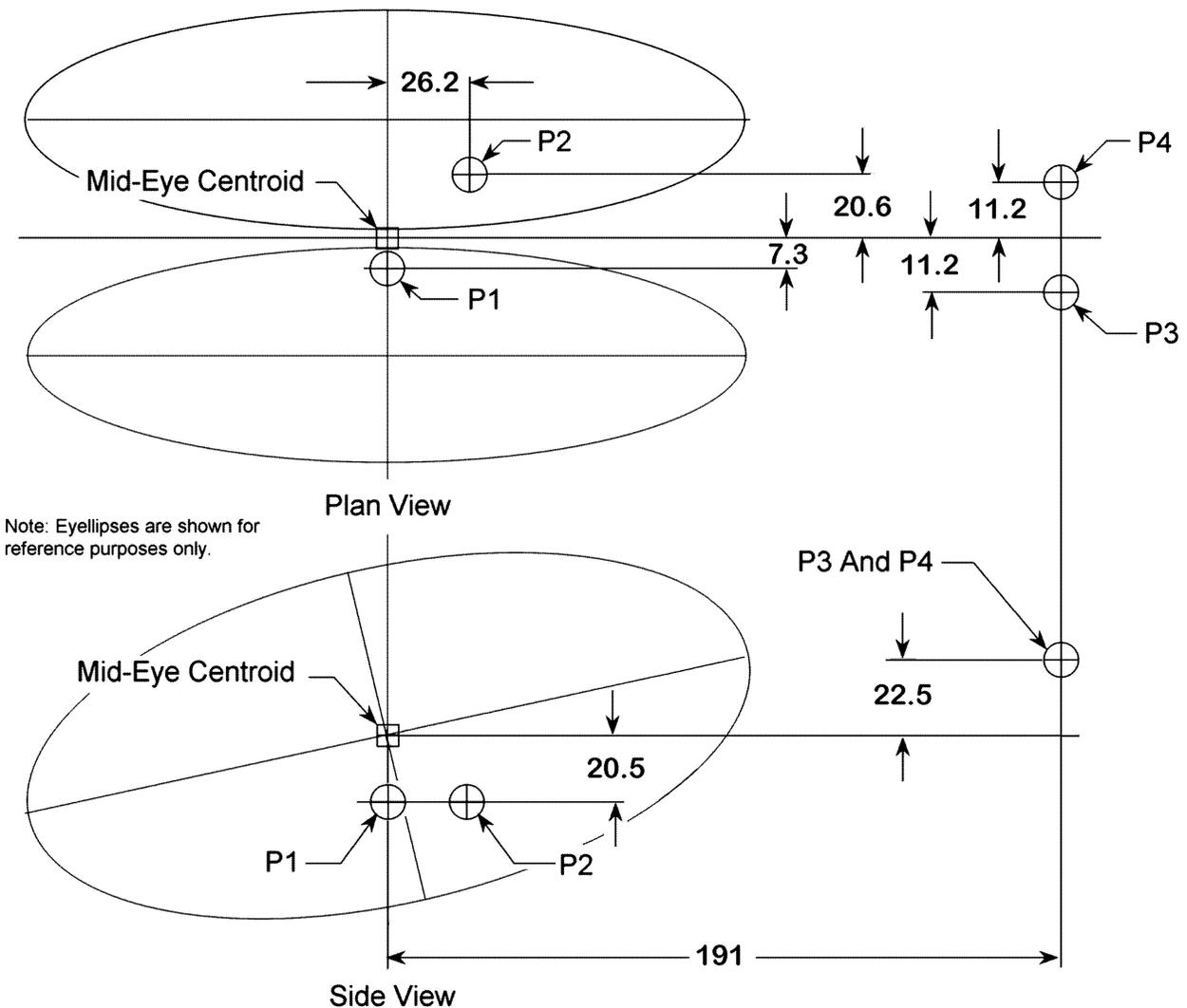
FIGURE 2—P-POINT LOCATIONS RELATIVE TO 95TH PERCENTILE EYELIPSE MID-EYE CENTROID WITH SEAT TRACK TRAVEL >133 mm
