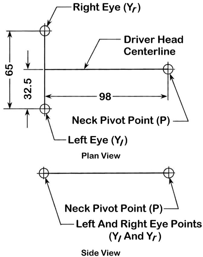
FIGURE 3—NECK PIVOT POINT AND ASSOCIATED EYE POINTS
