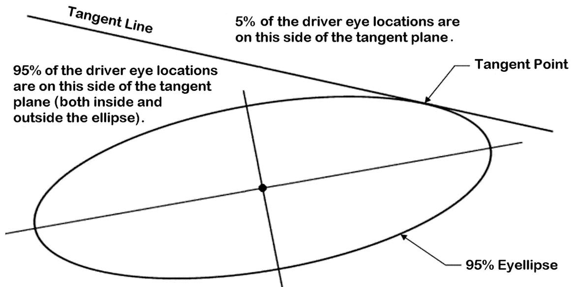
FIGURE D1—TWO DIMENSIONAL TANGENT CUTOFF DESCRIPTION.
