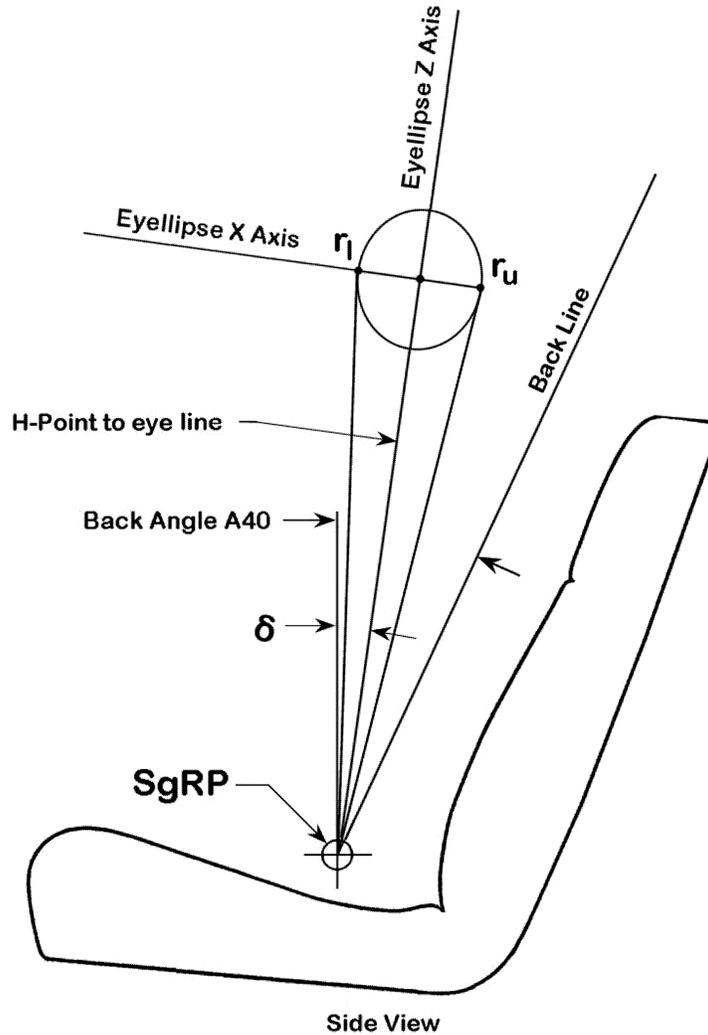
FIGURE C1—FIXED SEAT EYELLIPSE SIDE VIEW (X, Z)-AXIS AND AXIS ANGLE,  $\delta$ .
