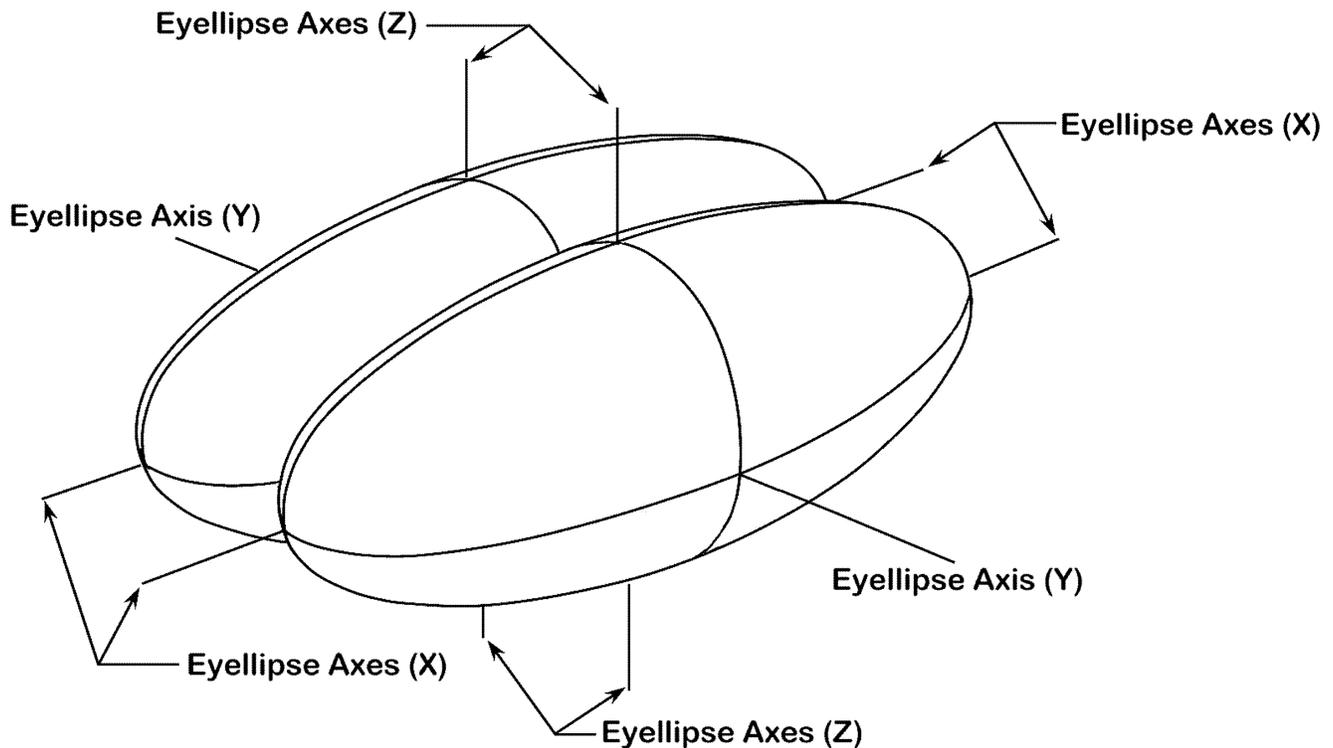
FIGURE 1—TYPICAL THREE-DIMENSIONAL TANGENT CUTOFF EYELLIPSES FOR THE LEFT AND RIGHT EYES
