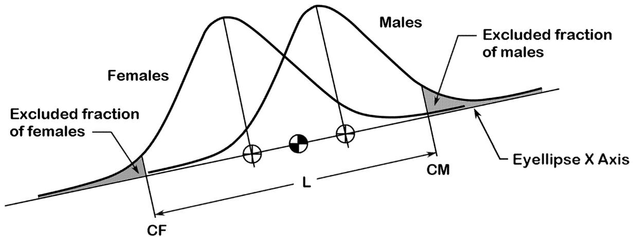
FIGURE A2—DETERMINATION OF EYELLIPSE X-AXIS END POINTS AND LENGTH
