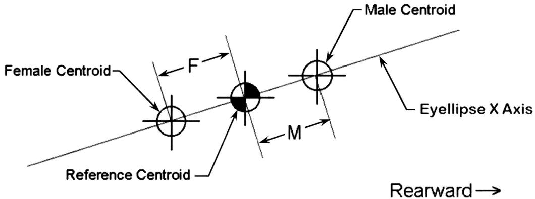
FIGURE A1—SIDE VIEW LOCATION OF THE MALE AND FEMALE EYE CENTROIDS RELATIVE TO THE REFERENCE CENTROID
